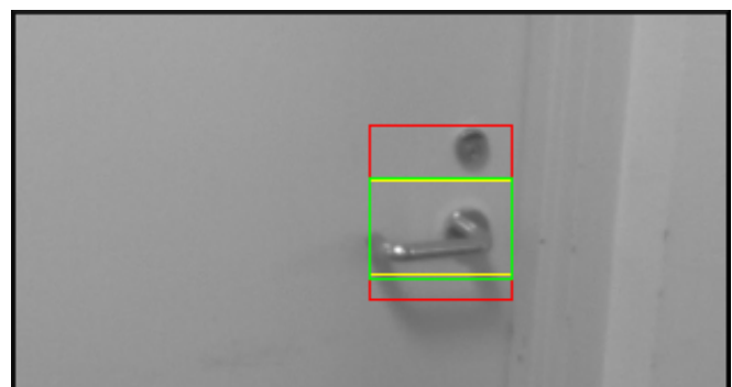
Fig. 5. Vision door handle detection. The green box is the final detection vote over seven frames, with intermediate detections represented by yellow boxes. The red box is a false detection filtered out by scale considerations.
