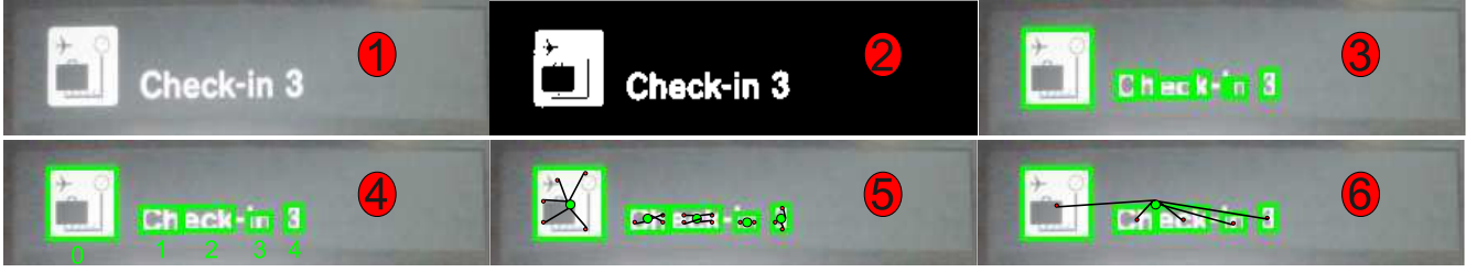
Fig. 1. Template processing. The input image 1 is binarized into image 2 with Otsu’s segmentation method. A region growing algorithm finds clusters of coherent colors in image 2 and outputs them in image 3. An agglomerative clustering algorithm groups the regions of image 3 into tokens in image 4. Image 5 shows the codebooks for each token of image 4. Image 6 shows the codebook for the entire sign from the tokens codebooks of image 4.
