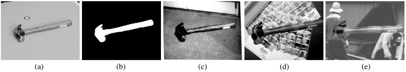
Fig. 3. Our synthetic data system: (a) Object view as seen by the capturing camera, with fiducial marking. (b) Mask extracted from the green-screen image. (c),(d),(e) Synthesized positive examples.
