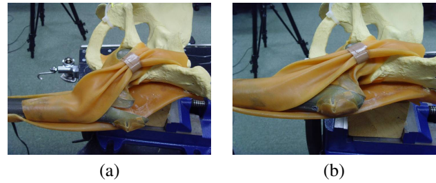
Fig. 12. Results of fracture reduction using the RCC-PA method: (a) before reduction and (b) after reduction.
