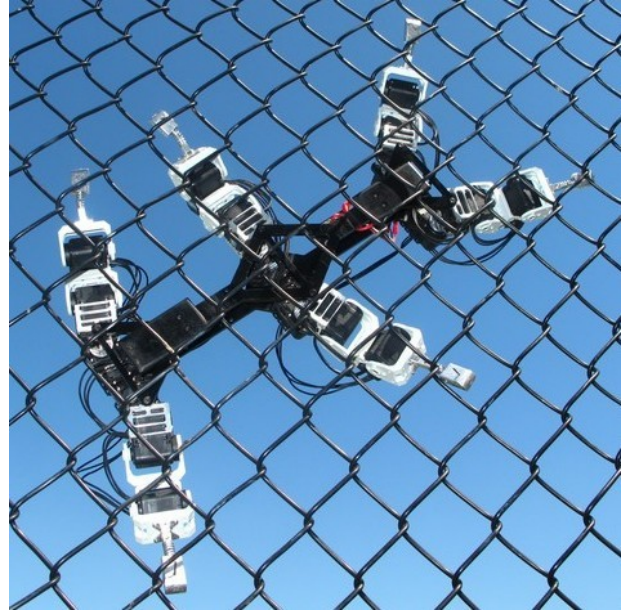
Figure 1. DIGbot is shown posed statically on chain-link fence. This 18-DOF hexapod is designed to perform complex maneuvers on a vertical surface using the Distributed Inward Gripping (DIG) attachment strategy.
