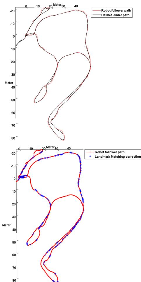
Fig. 10. Leader and follower paths for a typical run. Landmark match and hence pose correction locations shown on follower's path - note the jumps when there is a match after a longer interval.
