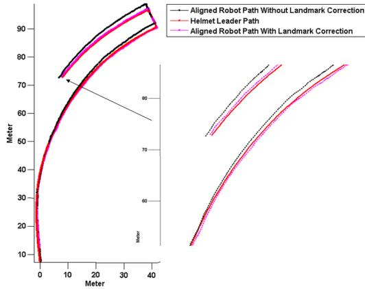
Fig. 3. Drift correction of visual odometry by matching against previously collected visual landmark database. The helmet operator walks along a marked path and collects the landmark database. The robot then loads in this database and runs visual navigation while being manually driven along the same path.
