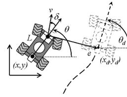
Fig. 4. Path following kinematic control for a car-like vehicle using lateral cross track error from reference path.
