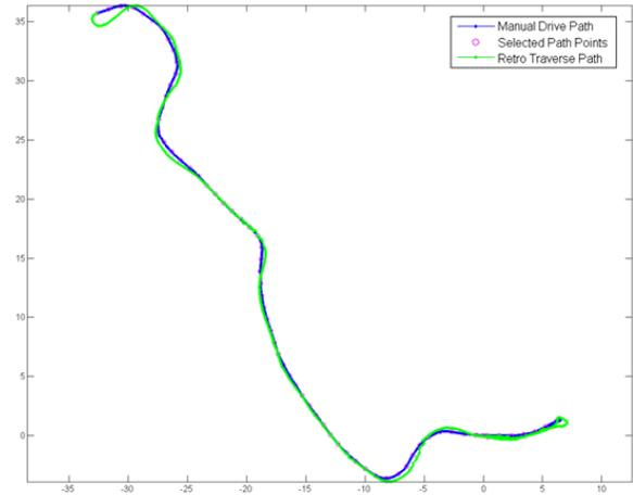
Fig. 9. Results of a typical retro-traverse run showing ground aligned 3 *DOF* pose derived from 6 *DOF* visual navigation pose output. The start (and return) position of the robot is at the origin for each plot. Note the path goes along a narrow sidewalk and over grass through bushes on either side. We have achieved similar results indoors in corridors as well.
