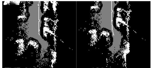
Fig. 7. Obstacle traversability maps based on dense stereo for a typical outdoor run. The black regions are unexplored or occluded, the gray region are best areas to traverse while lighter colors are increasingly hazardous with white being lethal.
