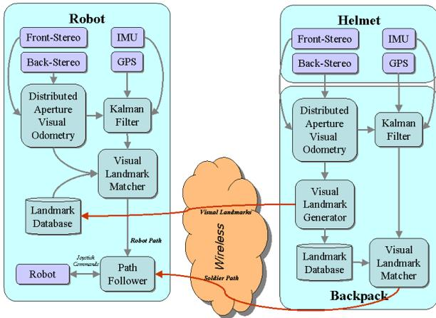
Fig. 2. A chart showing major hardware and software components of the *ViewTrek* leader-follower system. Hardware devices are purple, and algorithm blocks are blue. For retro-traverse the robot can be thought of as its own leader with no wireless networking requirement, but needing an additional software module for path reversal.
