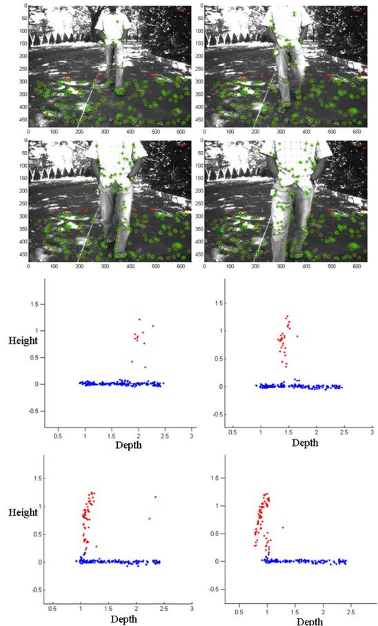
Fig. 6. Obstacle detection for hard stop using sparse 3D features. The top set of four images shows the Harris corner point features which satisfy the inlier and stereo matching criteria in red. The points that are closer than  $2.5m$  and used by the obstacle detector are circled in green. The bottom set of plots show the ground plane points in blue and the obstacle points in red.
