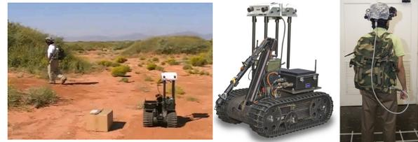
Fig. 1. (Left) The ViewTrek system in action during a leader-follower experiment. (Center) Mobile robot follower - The sensors are in the white boxes on the platform and the processor is in a black box visible on the side of the robot. (Right) Helmet leader - The cameras are visible on the sides of the helmet. The gray cable connects the sensors on the helmet to the processor inside the backpack.
