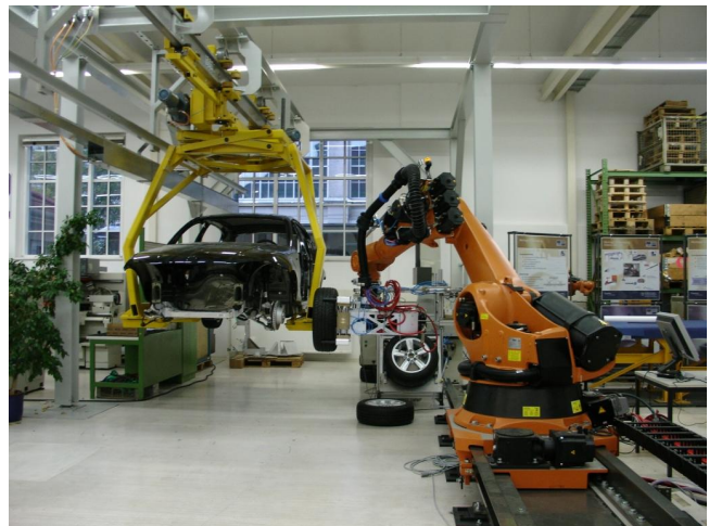
Fig. 1. Set-up at iwb for mounting wheels to a continuously moving car body
