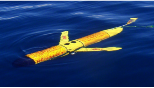
Fig. 1. The Slocum Glider, resting at the surface before diving.
