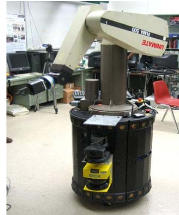
Fig. 1. Updated holonomic mobile robot system
