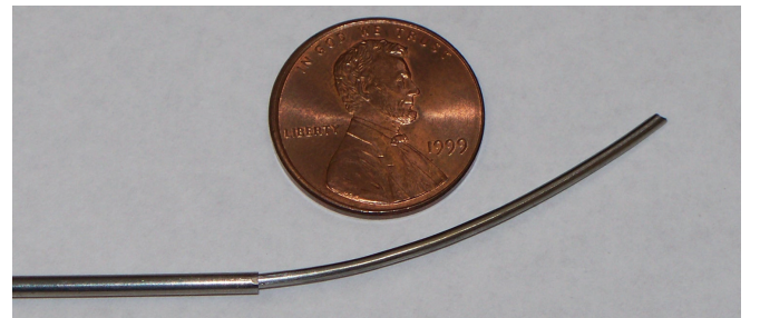
Fig. 3. Prototype active cannula consisting of a straight outer tube made of steel, and a precurved superelastic nitinol inner tube.
