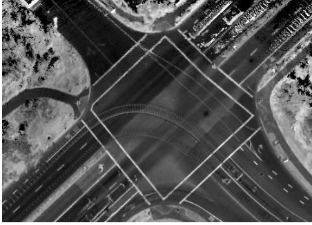
(b) Standard deviation of infrared reflectivity values.
