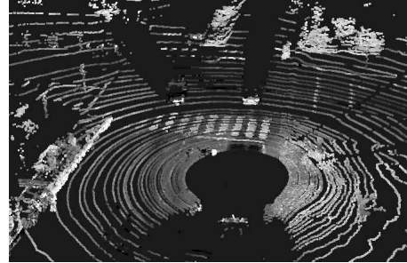
Fig. 3. Without calibration (a), each of the 64 beams has a significantly different response to reflectivity values. After calibration (b), the beams are much better matched.
