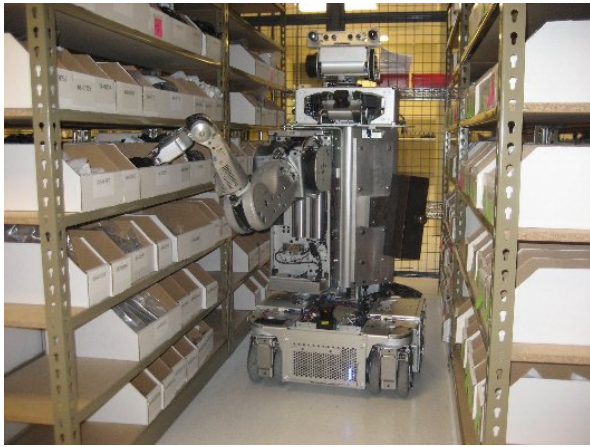
Fig. 1: The PR2 mobile manipulation platform.
