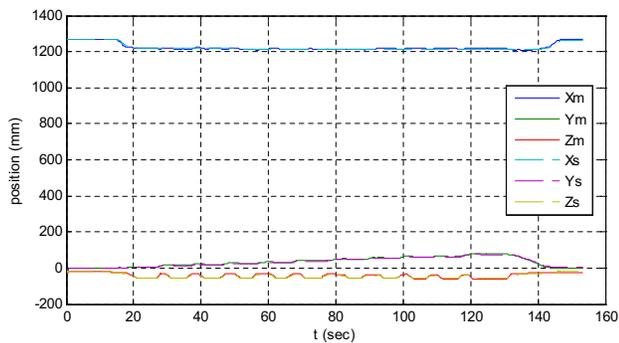
Fig. 8. The master-slave position tracking.
