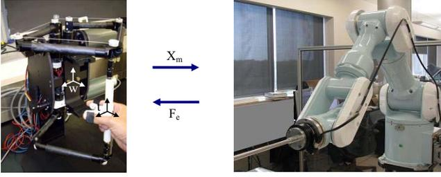
Fig. 3. Master-slave testbed: Left) Haptic wand, Right) Mitsubishi PA10 robot.
