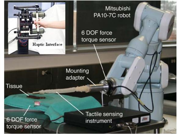
Fig. 4. Master-slave robotic setup palpating tissue.
