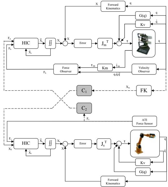
Fig. 6. The control system block diagram.
