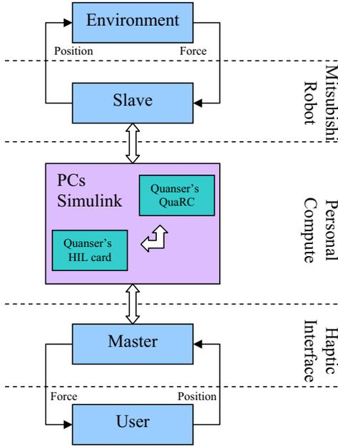
Fig. 5. Block diagram of the master-slave haptic teleoperation.
