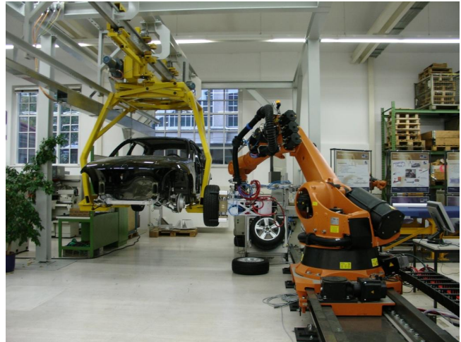
Fig. 1. Set-up at iwb for mounting wheels to a moving car body.
