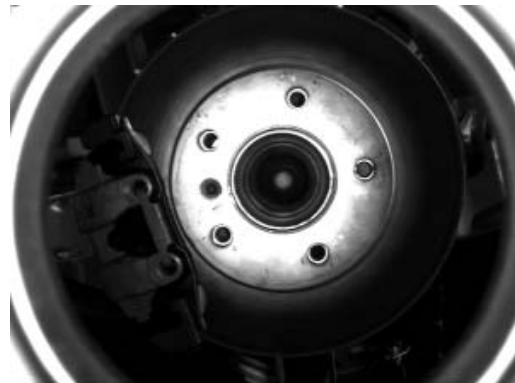
Fig. 3. Typical image of the robot mounted camera when measuring the pose of the wheel hub from greater distance.
