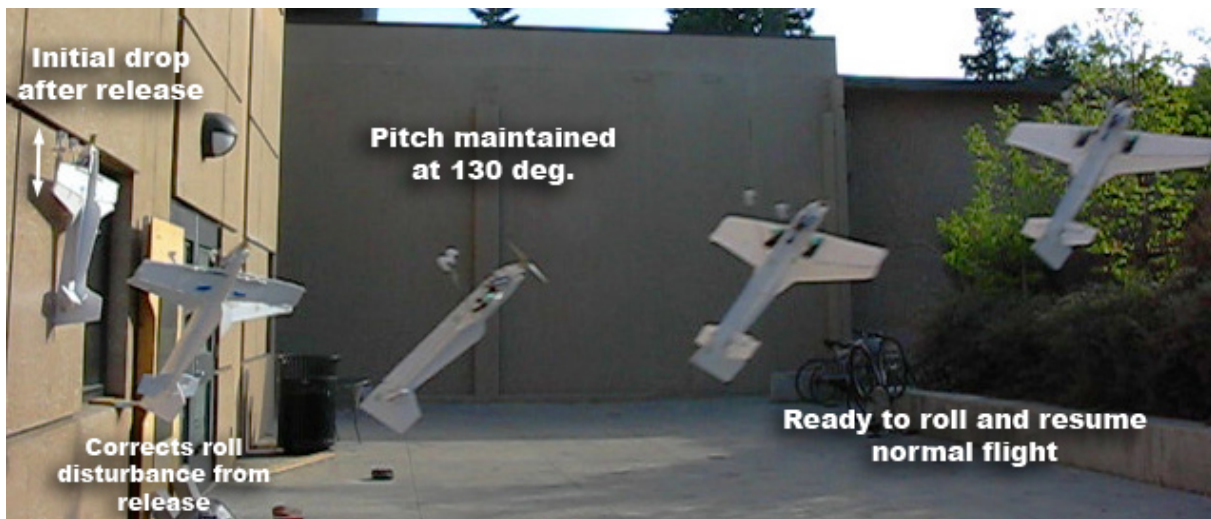
Fig. 5. A multiple-exposure photograph of the takeoff sequence. The airplane is originally at rest on the wall with ailerons and elevator ready for takeoff. The propeller is then commanded to a T/W ratio slightly less than 1.0; spines are released and the T/W ratio is increased to about 1.08 as the pitch angle is controlled to approximately 120 degrees from horizontal. Note that the spines have been intentionally released early in this example to clearly illustrate this step, but with ideal timing no vertical drop is observed.
