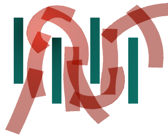
Fig. 6. An example solution to the path for the bending rectangle maze where a rectangle robot is required to bend through a simple maze.
