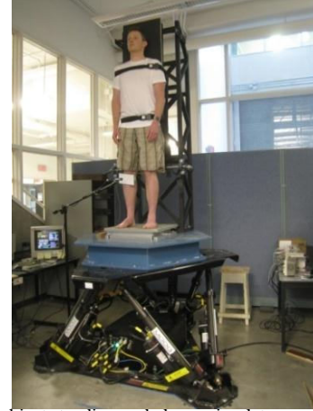
Fig. 2. Test subject standing on balance simulator.
