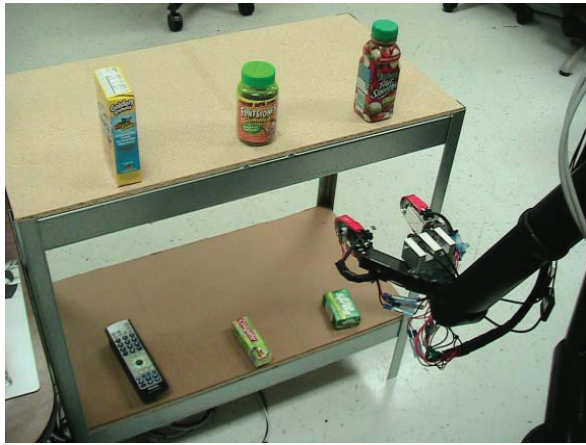
Fig. 1. Testing environment with 6DOF robotic arm with bi-level shelves and six ADL objects
