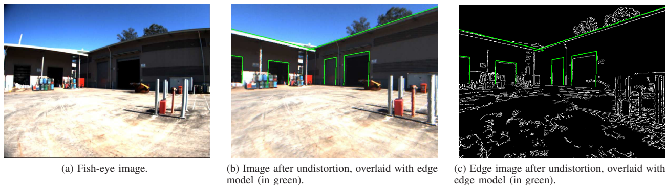
Fig. 8: Example of camera images and calibration.
