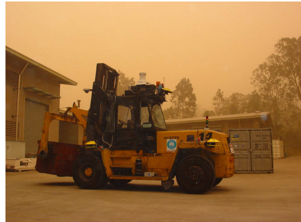
Fig. 1: The autonomous hot metal carrier.
