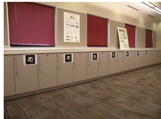
Fig. 2. The experimental setup. The black and white squares on the cabinets are the AR ToolKit markers used as landmarks.
