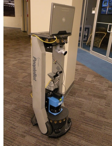
Fig. 1. The robot platform used for these experiments. The camera attached to the laptop is the one that is used to detect the AR ToolKit Plus markers.
