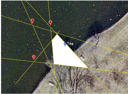
Fig. 9. Triangulation experiment: Cones of 45^\circ drawn around direction of maximum signal strength at locations A , B and C . Their intersecting polygon whose interior consists of possible location of the tag. The tag was actually placed at the location marked “Tag”.
