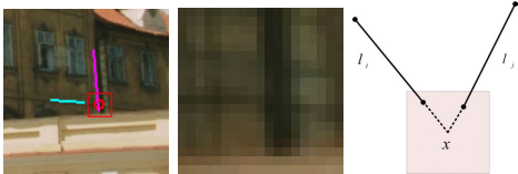
Fig. 1: (Left) An example of LICF. The line pair, colored in magenta and cyan, intersects in the circled position, with an intersection context bounded by the red box. (Middle) The zoom-in image of the intersection context. (Right) A model of LICF.
