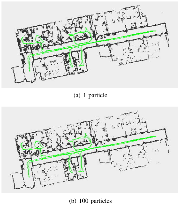
Fig. 9. Estimated map (black points) with the robot path (green curves) using 1 and 100 particles (raw sensor data), respectively.
