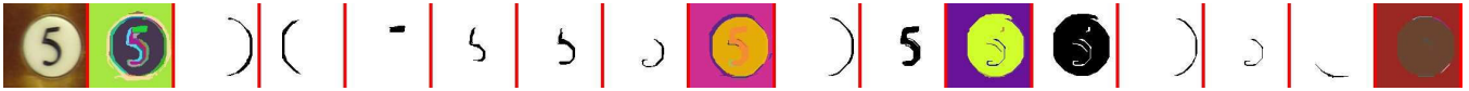
Fig. 7. Binarization step (best viewed in color). The first image is the original label. The other four non-binary images represent the output of the segmentation algorithm with four different parameter settings, with different colors corresponding to different segments. Each of these four segmentations is followed by binary images extracted from it using simple post-processing (discarding of segments that are deemed too large, too small, or circular). In this case only the second parameter setting produced a near-perfect segmentation of the character 5; however, all settings are needed for robust performance on varied elevator panels. Each of the obtained binarized images is then passed through OCR to extract a label.
