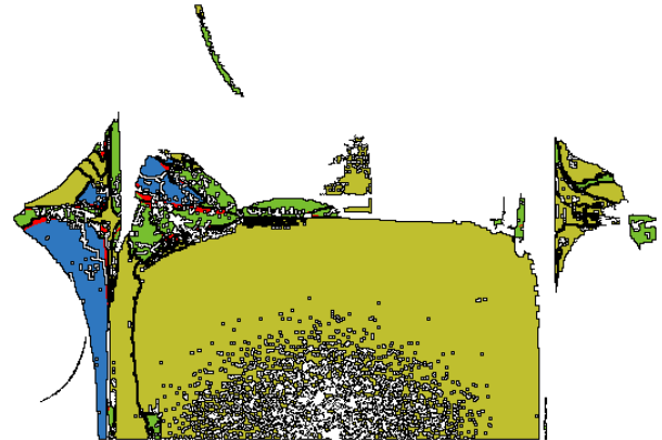
(c) The segmented range image with the patch types color coded. Note that the due to the large field of view the range image has spherical distortion when viewed as a rectangle. The black points represent the inter-patch boundary and are not used in LS fitting.
