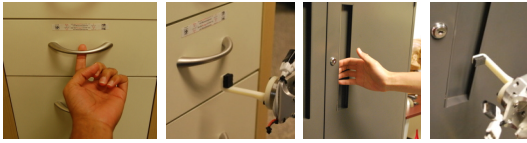
Fig. 3. Examples of a human using his hand as a hook, and corresponding orientations for the robot’s hook end effector.
