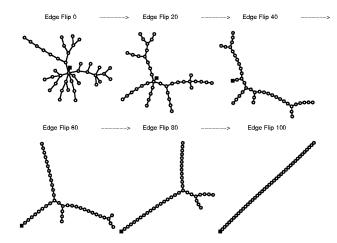
Figure 3. Selected iterations of a random tree graph with an external agent attached (square) running Protocol 1.
