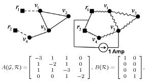
Figure 2. Left: Network graph with external (control) agents  $r_1$  and  $r_2$  attached to agents  $v_1$  and  $v_4$  respectively, leading to an altered Laplacian  $A(\mathcal{G}, \mathcal{R})$  and input matrix  $B(\mathcal{R})$  of model (2). Right: Equivalent electrical network. The potential difference  $V_{v_3} - V_{\mathcal{R}}$  is the effective resistance between  $v_3$  and common resistor node  $\{r_1, r_2\}$ .
