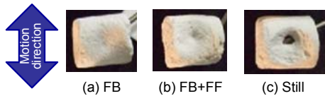
Fig. 14 Destruction results of model stones by HIFU
