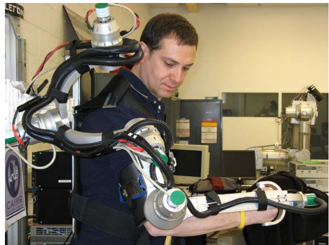
Fig. 1. The MGA Exoskeleton has six degrees of freedom and force/torque sensors mounted on both the upper arm and handle.
