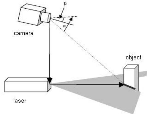
Fig. 1. Geometric configuration of a laser line striper.
