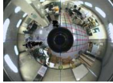
Fig. 1. The omnidirectional image of the cross-stripes on the floor. This image is used for deciding the parameters.
