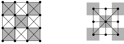
Fig. 3. Grid layout over map grids. Graph nodes and edges are black, map grids are gray and white. Field-D* places nodes at grid corners (left), while A*, D*, and D* Lite traditionally place nodes at grid centers (right).
