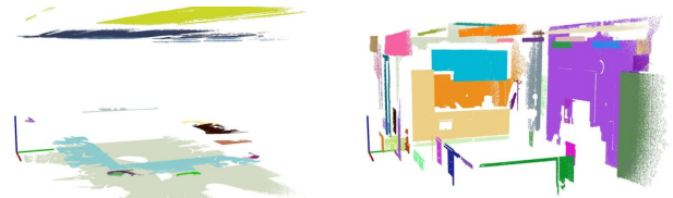
Fig. 6. Left: all horizontal planes found in the scene; right: all vertical planes found in the scene.
