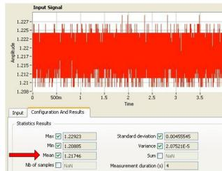
Fig. 12. Y axis values of the accelerometer at 40°
