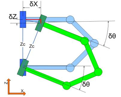
Fig. 5. The error on the placement of the base generates a relative error on the manipulator
