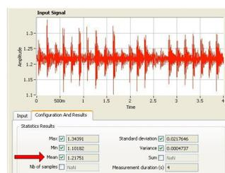
Fig. 13. Y axis values @ 40° & 6Hz normal amplitude vibration
