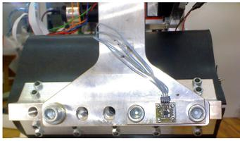
Fig. 11. The inclinometer board installed on the upper link
