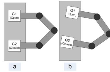
Fig. 1. Errors on the positioning of the base of the robot cause error on the manipulator of the robot
