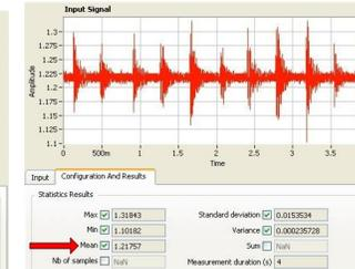
Fig. 14. Y axis values @ 40° & 3Hz normal amplitude vibration
