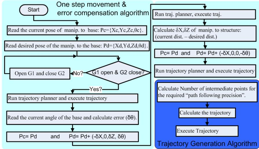
Fig. 4. Self calibration algorithm
