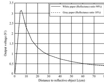
Fig. 9. The output “voltage” of the Sharp sensor against the “distance to a gray & a white paper”
