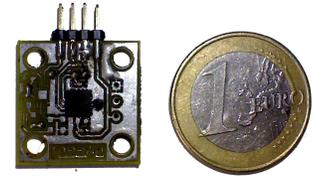
Fig. 10. The accelerometer board developed at ISR
