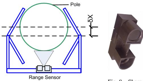
Fig. 7. Schematic of the gripper distance error compensation
