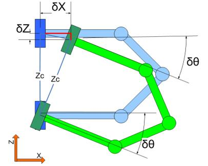
Fig. 5. The error on the placement of the base generates a relative error on the manipulator
