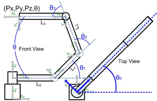
Fig. 3. Schematic of the 4 DOFs serial climbing mechanism
