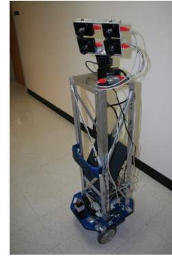
Figure 7. The quad stereo system on a mobile platform used in Sec. 4.4.
