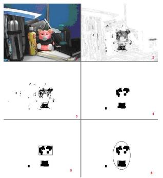
Fig. 2. Illustration of the four steps in rough detection. The first image is the input image. The second is the back projected image. The third is the binary image after thresholding. The fourth is the binary image after morphological filtering. The fifth is the detected blobs in the binary image. In the sixth image, the ellipse is the detected precise result from the corresponding rectangle. The grayscale image are **NOT**ed for easier viewing.
