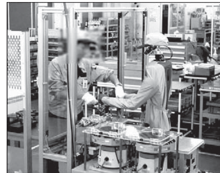
Fig. 1. Cooperative work of SP-02 with a human worker in a cell workspace
