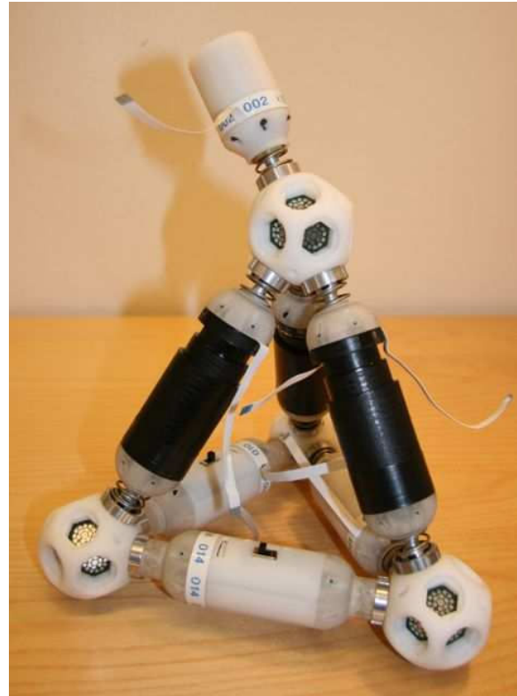
Fig. 1. An example of the Odin robot in a tetrahedron configuration with a rigid base of battery modules and a flexible top of telescoping modules. A wireless module is connected to the top node.
