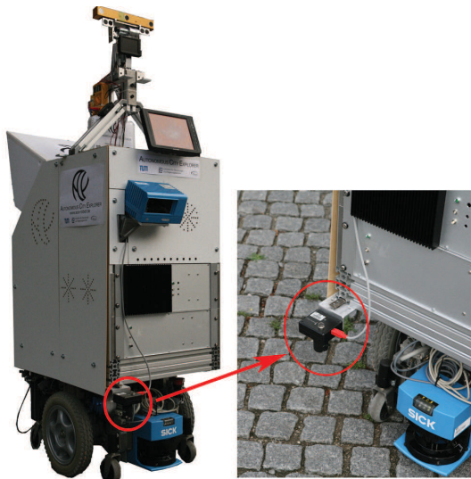
Fig. 1: ACE robot and the camera for visual odometry
