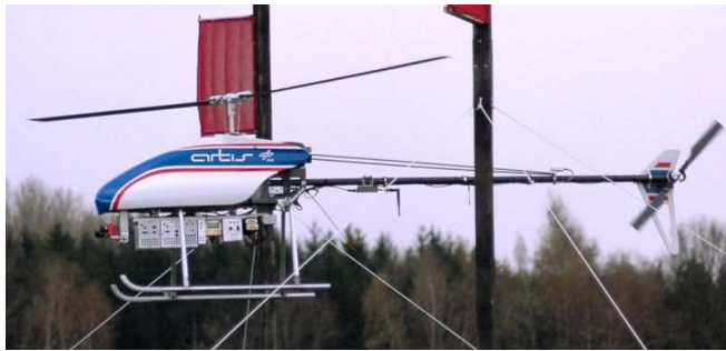
Fig. 8. The helicopter ARTIS flying through obstacle posts.
