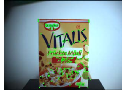
Fig. 1. Image used for evaluation of the scale coverage of the SIFT descriptor. For this image, 284 feature points were calculated by the Harris corner detector, using a quality threshold of 0.01. The computed feature points are marked by the green dots.
