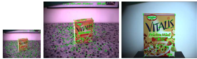
Fig. 4. Images used for testing the performance of the extended Harris-SIFT features. The computed feature points are marked by the white dots. Left: view corresponding to a scale of 0.32 relative to the training view, with 438 computed feature points. Middle: view corresponding to a scale of 0.64 relative to the training view, with 500 computed feature points. Right: training view, with 284 computed feature points.
