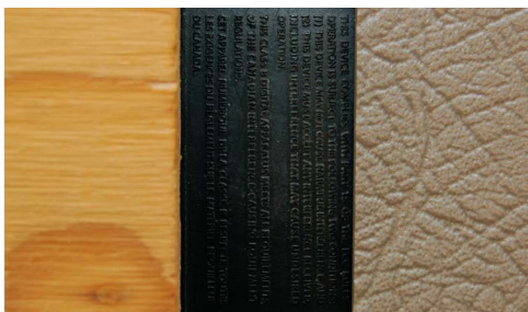
Fig. 8. The three surfaces that were tested with the teleoperation system: unfinished plywood, hard plastic embossed with text, and textured vinyl.
