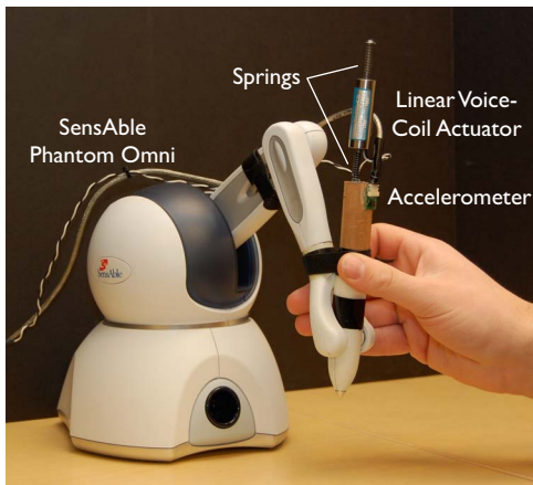
Fig. 3. The haptic interface we developed to test the efficacy of the proposed approach. The standard stylus of a SensAble Phantom Omni was replaced with a custom handle for attachment of a dedicated vibration actuator and an accelerometer.
