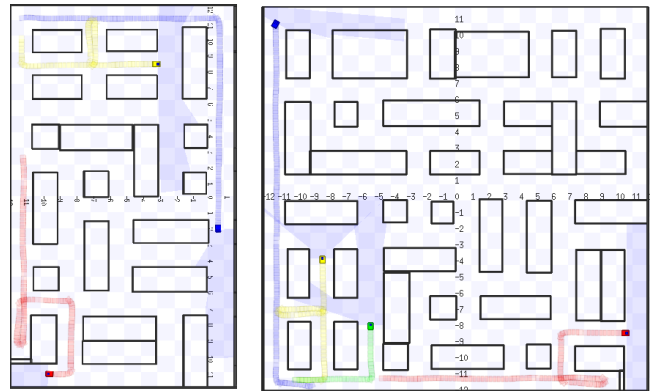
Fig. 6. Maze No.2(left), 82 nodes, 3 robots exploring. Maze No.3 (right), 135 nodes, simulation, 4 robots exploring
