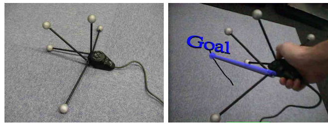
Fig. 6. Pointing device which can be tracked via motion-capture, and its appearance in the augmented reality system.
