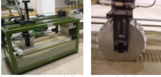
Fig.6 Wheel-soil interaction test bed and experimental wheel. cal metal wheels with different radii, widths and lugs were used, as shown in Table I, where n_L is the number of wheel lugs.
