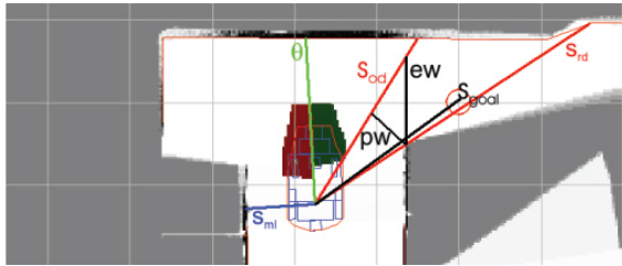
(b) Evidence grid representation of the environment (cf. Section IV) along with a centered and upward facing bounding-polygon of the wheelchair. The target p_g is depicted as a circle.
