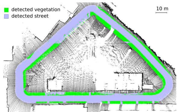
Fig. 7. Mapping of a large outdoor environment. The laser was tilted at a fixed angle of 20 degrees while the robot was moving. The figure shows a 2D projection of the 3D map.
