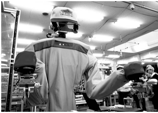
Fig. 1. SP-02 robot with humanoid upper-body for cell production line
