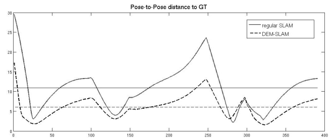
Fig. 5. [Artificial Dataset] Distance to GT best fit. Average regular estimation: 10.8602. Average DEM approach: 6.0338. X-axis shows the pose, Y-axis shows meters.
