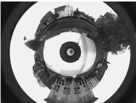
Fig. 1. Outdoors omnidirectional image taken from the roof of the vehicle
