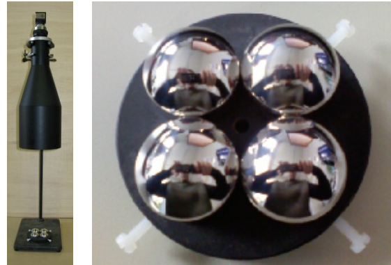
Fig. 1. Our sensor: orthographic camera, parabolic mirrors, 90 cm height
